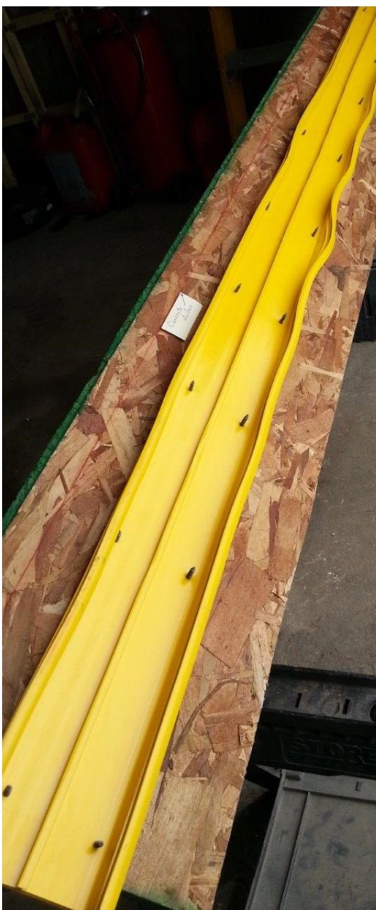
RibLok attached to form sample.
